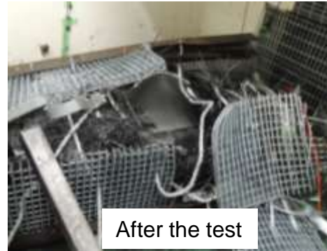
Maximum filling pressure : 82 MPa Internal volume: ~200 L
