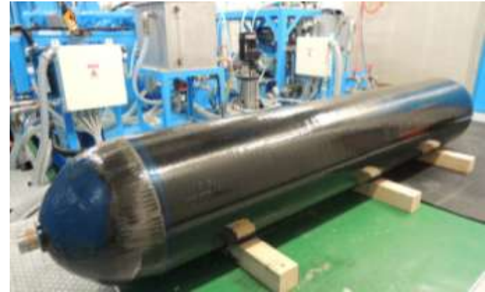
Maximum filling pressure : 82 MPa Internal volume: ~200 L
