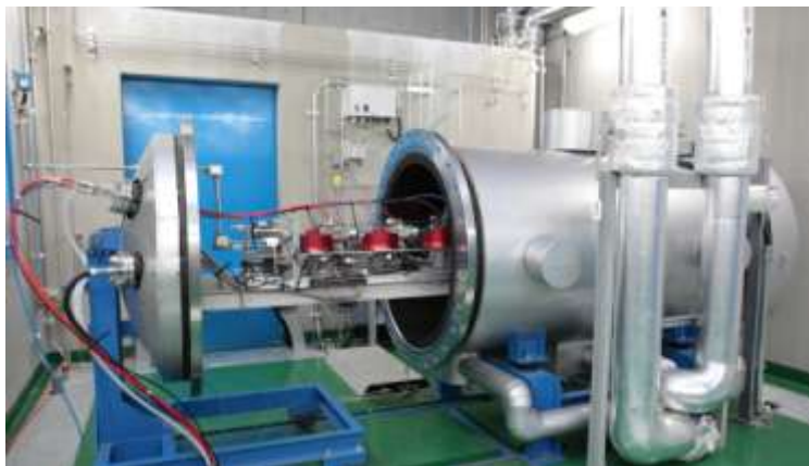
40,000 cycle durability test in 2012 The ball valves were commercialized in 2012. Cross section
