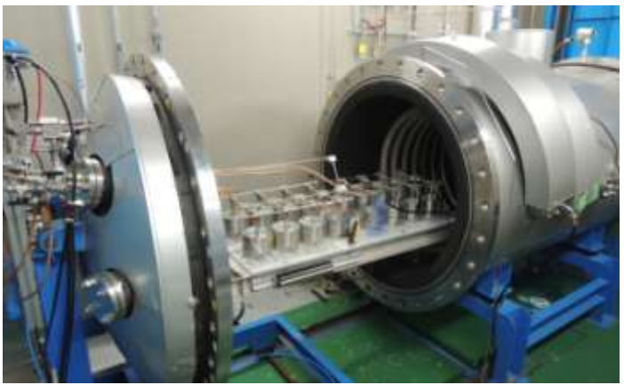
16 sample holders in the explosion resistant chamber
