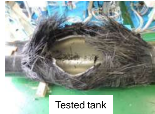
Maximum filling pressure : 82 MPa Internal volume: ~200 L
